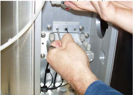
3. Disconnect air lines (push collar in to release).
