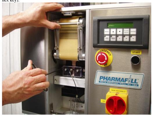
2. Remove Rear Mark Sensor Block with fiber optic (1/8 hex key).
