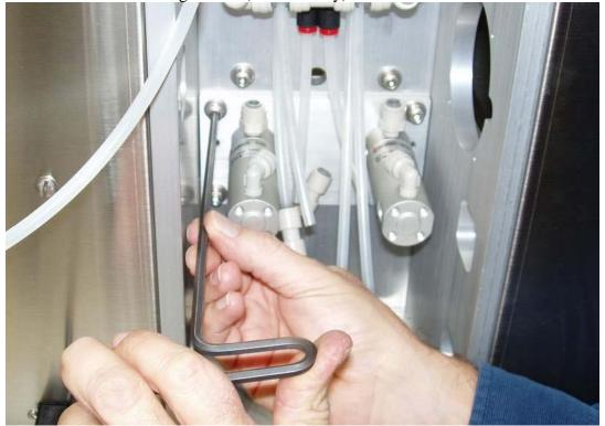
5. Support assembly while removing last screw.
