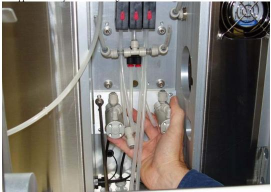
6. Lift air lines out of the way.
