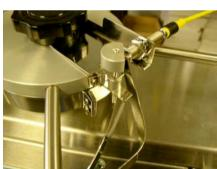
Spring loaded deflector guide- pushes pills toward the inside edge of the rim. Spring tension is adjusted by hooking the end of the spring in a different hole in the top edge of the guide. Bend the guide tip as required to get the most desirable product control. As the deflector moves so does the AVC target which will turn on/off the vibrator accordingly.
