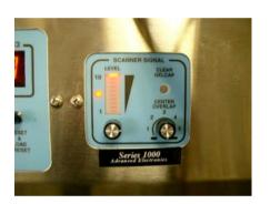
Scanner signal display panel. 10 segment bar graph display shows scanner signal level. It reacts quickly as pills pass through the scanner beam. An adjustment knob below display sets the maximum signal at 9-10 level for normal operations. the Clear Gelcap Center Overlap circuit makes it possible to count clear gel caps accurately. Always set at minimum (CCW) when counting pills that are not perfectly clear.
