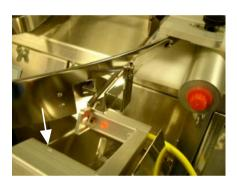
Flow correction guide - 2 part stainless steel assembly that keeps odd shaped pills from falling from the glass plate at an undesirable angle. It attaches to the rim spoke hardware and positions a wedge shaped edge next to the glass. This wedge presents a square edge which causes the pill to fall straight through the centerline of the scanner. The dot (white arrow) over the scanner photocell shows the centerline of the scanner beam from the red LED to the photocell.
