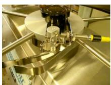
Automatic Vibrator Control (AVC) sensor- The yellow cable leads to an inductive sensor that is aimed at an aluminum half-round block referred to as the AVC target. When the sensor detects the target, a light at the rear of the sensor goes on and the vibrator turns off. Adjust the target so when the spring loaded deflector guide is moved by a body of pills on the glass the target moves in front of the sensor. This will keep the glass plate from being overloaded by pills.
