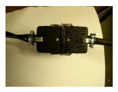
Multi-pin connector- Connect the line power cable from 115 VAC outlet to this connector to use the TC2 as a table top semi automatic machine. This large connector serves the purpose of several circuits that are part of the TC2 when used in a fully automatic ABF2 set up and are not used for semi automated operations.
