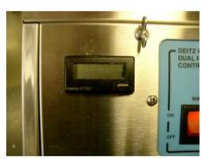
LCD counter. This small self contained counter totals the number of bottles filled during a filling operation period. A reset button clears the readout when pushed. The counter will increase by one a unit each time the diverter head changes filling stations which during production should equal a filled bottle.
