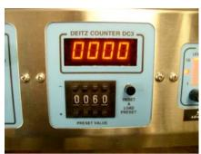
DC3 electronic counter. Readout shows how many pills are counted by the scanner. The push button register below display is set for the number of pills to be counted into the bottle. The push button reset clears the readout to 0000. Do not spray this panel to clean. Do not allow fluids to drip inside the registers.
