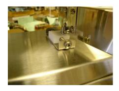
Rim location adjustment. This combination pin and fork align the rim and the product guides with the scanner and diverter head when the machine is reassembled after cleaning. Care must be taken when installing the rim to be sure the fork is not deformed by misalignment of the fork and pin. To move the rim CW/CCW on it's center axis adjust the screw while observing the pills as they drop from the glass plate through the scanner.
