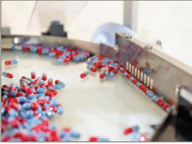
Proprietary Airguide System automatically sets pills onto a single layer and guides their flow into the center of the counting mechanism for proper presentation to the counting sensor.
