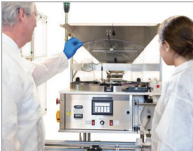
No change parts needed for easy setup, usage and breakdown without tools. Complete product changeovers in less than five minutes - including testing.
