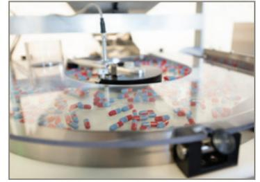
Deitz counting technology allows sensor adjustments to suit the solid dosage form. It even flashes an alert if cleaning may soon be needed.
