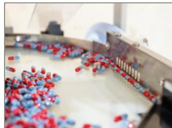
Proprietary Airguide System option automatically sets pills onto a single layer and guides their flow into the center of the counting mechanism for proper presentation to the counting sensor.
