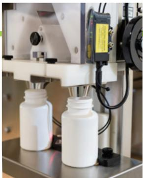
Smart bottle sensing option verifies when the bottle is ready for filling and automatically stops operation if a bottle is missing.
