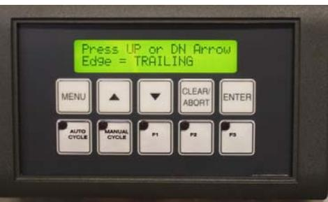
LEADING means the registration signal will be turned on as the leading edge of the seam is detected (pouch-to-seam). This is the default selection.
