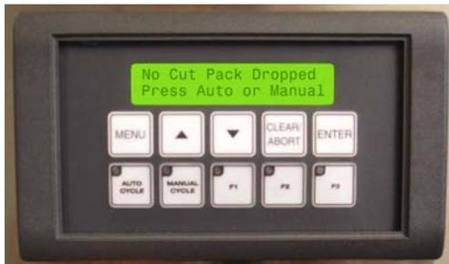
7. The control panel will display “No Cut Pack Dropped” when the CUT PACKET SENSOR in the Exit Tube does not immediately detect a cut packet dropping through after a cut. The operator must press CLEAR/ABORT and correct the problem.
