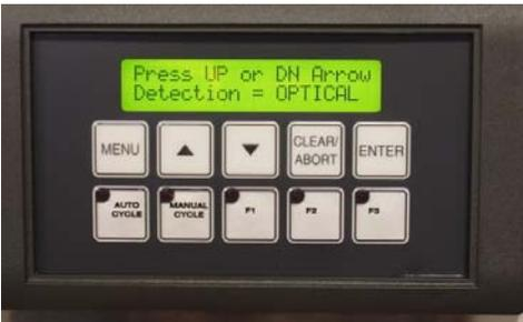
Seam Detection: OPTICAL (up) or ROLLER (down)
