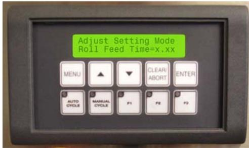
6. The fifth setting is “Roll Feed Time”. This is the duration of each advance action of the Roll Feed, which controls the length of roll feed. Adjust this value by using the UP or DOWN arrow keys. Press ENTER to accept the value and move to the next setting. Refer to document TN0092.
