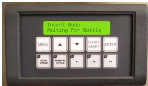
4. The control panel will display “Waiting for Bottle” when there is no bottle at the START SENSOR. A cycle will start as soon as a bottle is detected.
