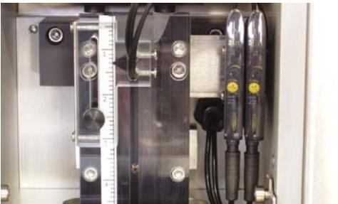
4. Cut Length Sensors Assembly as mounted on Drop Chute.
