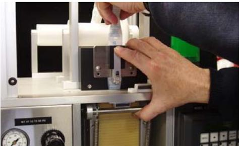
To feed the strip into the guides, open the door and press the top of the roller lever while lifting the belt feed release bar.
