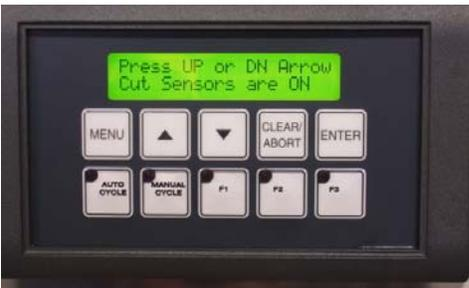
Cut Sensors ON/OFF (up/down)
