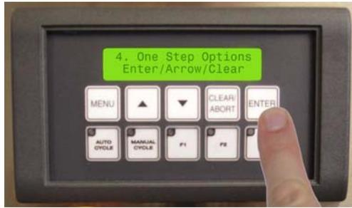
1. The One Step mode lets you control each part of the inserting process individually.
