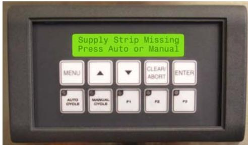
6. The control panel will display “Supply Strip Missing” when there is a no strip in front of the SUPPLY STRIP SENSOR in the Upper Guide Block. The machine will not cycle. When the supply strip is restored, the cycle will resume.
