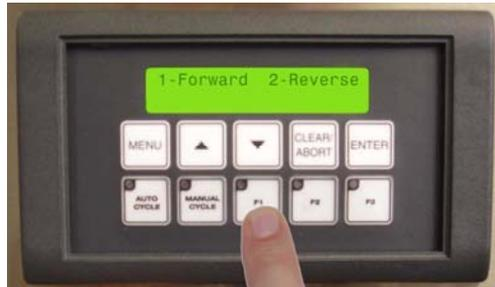
2. Select one of the options by using the “F” keys. Press F1 to move the belt forward (down).
