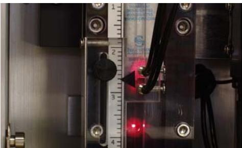
The upper sensor is the SHORT sensor. The lower sensor is the LONG sensor. Prior to starting a cut and feed cycle, the Short sensor must detect the lowest edge of the strip, while at the same time the LONG sensor must NOT detect anything. If these conditions are not met, the cycle is aborted and the type error is reported on the HMI.
