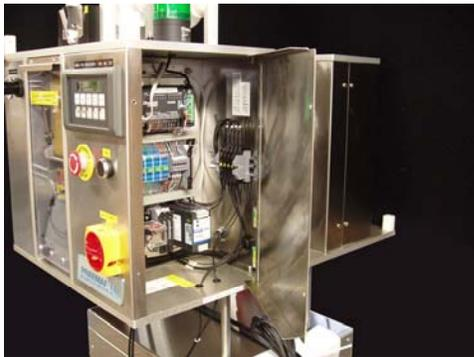
6. Hinges added to right side access cover for ease of service and adjustment.
