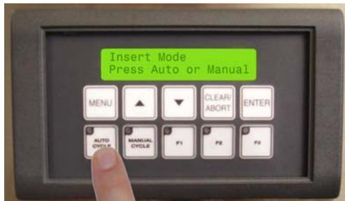
3. To automatically cycle whenever a bottle is present, press AUTO CYCLE. The machine will cycle when a bottle is present at the start sensor and all proper conditions are met. This is an alternate contact button. Press once to turn it on; press again to turn it off.
