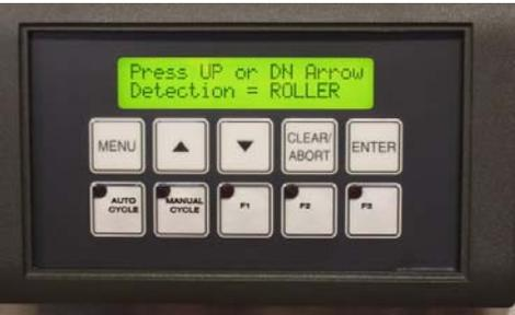
ROLLER uses the roller and proximity sensor which is located above the belt feed. Best for packets without the punched hole in the seam. May also be used for pack with the hole. Press the DOWN arrow.
