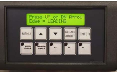
Edge Detection: LEADING (up) or TRAILING (down). Allows the use of two different ranges for offset values, to find the right cut location and to avoid double feeds. Change this setting if you have difficulty getting the cut in the middle of the seam, such as when the offset value is close to zero or very high. Also change it if you get double feeds
