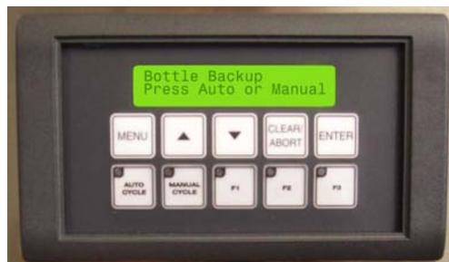
5. The control panel will display “Bottle Backup” when there is a bottle in front of the BACKUP SENSOR. The machine will not cycle. Once the backup is cleared, the cycle will resume.
