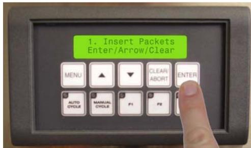
Insert Packets mode is used to manually or automatically run the machine.
