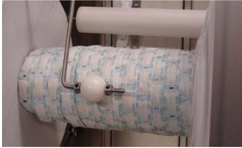
5. Low Roll Sensor Arm – detects when the supply roll is more than half empty, briefly causing the yellow light to flash and a message be displayed, once every 5 seconds.
