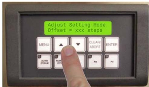
2. The first setting is “Offset”. This number controls how far the packet strip is advanced after the PACKET MARK SENSOR detects the registration mark. Adjust this value by using the UP or DOWN arrow keys. Press ENTER to accept the value and move to the next setting. Refer to document TN0097. (Units = step motor pulses, Range = 0 to 999)
