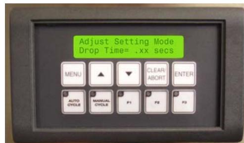
4. The third setting is “Drop Time”. This is the time needed for a packet to drop from the cutoff knife to the bottle. Adjust this value by using the UP or DOWN arrow keys. Press ENTER to accept the value and move to the next setting.
