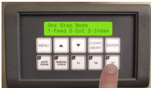
4. Press F3 to control the bottle indexing function. This is an alternating function. Press once to advance all the bottles by one position. The next bottle is now in the filling position. Press again to release the first bottle. This allows you to check that the position of each Bottle Gating Stop is correct.
