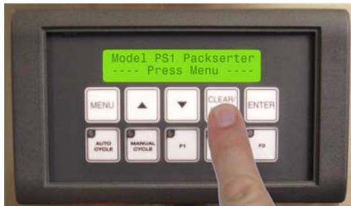
8. Press CLEAR/ABORT to exit Adjust Settings mode at any time and return to the top menu.
