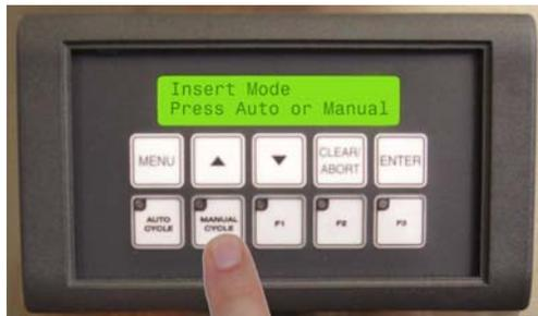
2. To cause the machine to make one cycle, press MANUAL CYCLE. The machine will make one cycle even if there is no supply strip loaded. This is a momentary contact button. It may be held down to cycle continuously.
