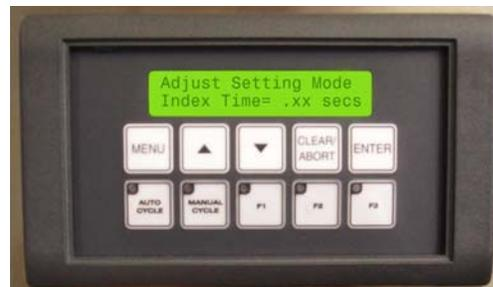
5. The fourth setting is “Index Time”. This is the time needed for the bottles to advance one position on the conveyor. Adjust this value by using the UP or DOWN arrow keys. Press ENTER to accept the value and move to the next setting.
