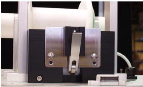
3. Roller Proximity Sensor - for Strip Presence sensing (dynamic only) and Seam Detection for cut-off registration (user option)
