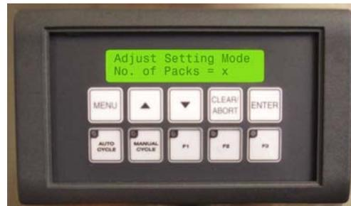
3. The second setting is “No. of Packs”. This is the number of cut packets to be dropped into each bottle. Adjust this value by using the UP or DOWN arrow keys. Press ENTER to accept the value and move to the next setting.
