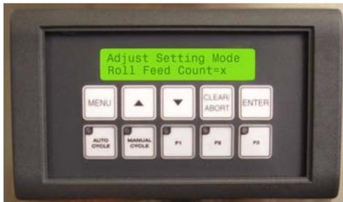
7. The sixth setting is “Roll Feed Count”. This is the number of advances actions that will made in one cycle. Adjust this value by using the UP or DOWN arrow keys. Press ENTER to accept the value and return to the MENU screen.
