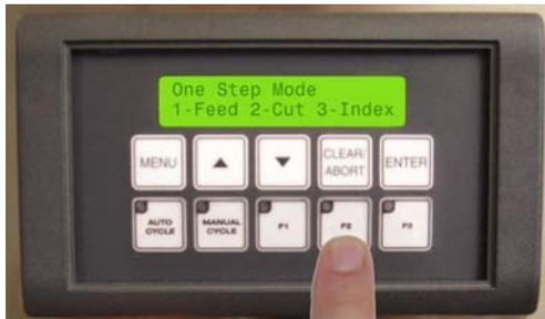
3. Press F2 to control the cutoff knife. This is an alternating function. Press once to close the knife. Press again to open the knife. This allows you to check the performance of the cutting action.
