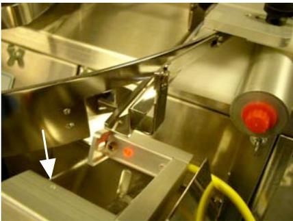
Flow correction guide - 2 part stainless steel assembly that keeps odd shaped pills from falling from the glass plate at an undesirable angle. It attaches to the rim spoke hardware and positions a wedge shaped edge next to the glass. This wedge presents a square edge which causes the pill to fall straight through the centerline of the scanner. The dot (white arrow) over the scanner photocell shows the centerline of the scanner beam from the red LED to the photocell.
