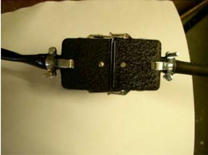
Multi-pin connector- Connect the line power cable from 115 VAC outlet to this connector to use the TC2 as a table top semi automatic machine. This large connector serves the purpose of several circuits that are part of the TC2 when used in a fully automatic ABF2 set up and are not used for semi automated operations.
