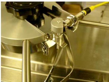
Spring loaded deflector guide- pushes pills toward the inside edge of the rim. Spring tension is adjusted by hooking the end of the spring in a different hole in the top edge of the guide. Bend the guide tip as required to get the most desirable product control. As the deflector moves so does the AVC target which will turn on/off the vibrator accordingly.
