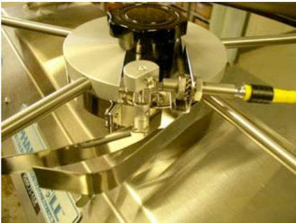
Automatic Vibrator Control (AVC) sensor- The yellow cable leads to an inductive sensor that is aimed at an aluminum half-round block referred to as the AVC target. When the sensor detects the target, a light at the rear of the sensor goes on and the vibrator turns off. Adjust the target so when the spring loaded deflector guide is moved by a body of pills on the glass the target moves in front of the sensor. This will keep the glass plate from being overloaded by pills.
