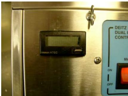
LCD counter. This small self contained counter totals the number of bottles filled during a filling operation period. A reset button clears the readout when pushed. The counter will increase by one a unit each time the diverter head changes filling stations which during production should equal a filled bottle.
