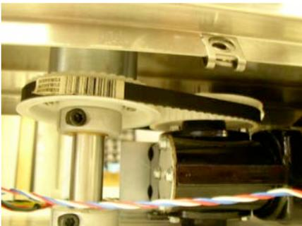
Turntable drive assembly- picture of the motor and turntable support hub from inside the TC2. A belt connects between two plastic gear belt pulleys. To adjust belt tension loosen the gear motor mounting bolts from under the TC2 center section. The belt is adjusted OK if you can easily move the center unsupported section of the belt about 1/2" in and out. To prevent failure of the plastic pulley do not over tighten the belt.
