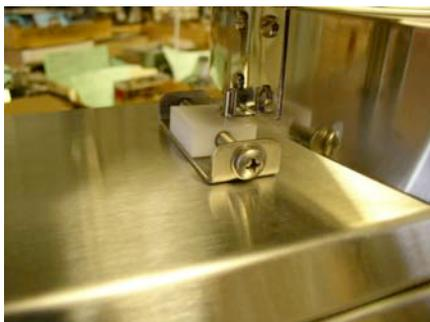
Rim location adjustment. This combination pin and fork align the rim and the product guides with the scanner and diverter head when the machine is reassembled after cleaning. Care must be taken when installing the rim to be sure the fork is not deformed by misalignment of the fork and pin. To move the rim CW/CCW on it's center axis adjust the screw while observing the pills as they drop from the glass plate through the scanner.
