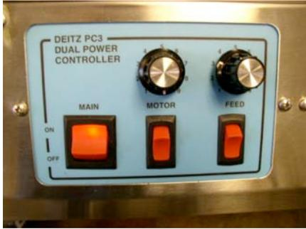
PC3 power control module. Switches turn on the main, motor (turntable) and feeder (vibrator) power. Feeder will not turn on if motor is off. Motor speed and vibration intensity is controlled by the adjustment knobs. Fuses located on the interconnection panel inside the TC2 protect these circuits.
