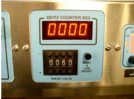
DC3 electronic counter. Readout shows how many pills are counted by the scanner. The push button register below display is set for the number of pills to be counted into the bottle. The push button reset clears the readout to 0000. Do not spray this panel to clean. Do not allow fluids to drip inside the registers.
