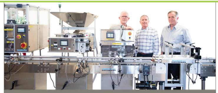
Pharmafill powered conveyors feature a modular design with standard lengths of three and six feet for smooth, automated bottle movement from one filling or packaging machine to another.
