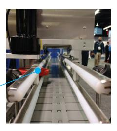
This spacer wheel (optional) slows the bottle speed to create a gap between bottles for easier labeling, capping and neck banding and/ or to help downstream equipment keep pace.
