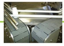
Deitz engineers set a rotary turntable between two conveyors to transfer bottles around corners.
