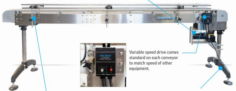
Adjustable rail system with dual guide rails as standard permits quick changes to height and width. Smooth plastic
