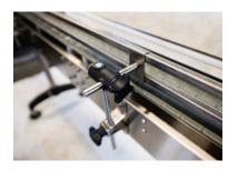
protects bottles from any rail contact. Pre-threaded clamping brackets allow spacing wheels, turntables, reject stations and other attachments to be quickly moved without drilling holes.
