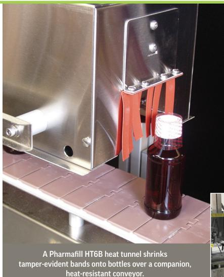
The Pharmafill HT6B Heat Tunnel automatically shrinks tamper-evident bands and sleeve labels onto bottles and other containers with a consistent – perfect – seal every time. How? A proprietary engineering advance directs an energy-efficient blend of convection and radiant heat toward the bottom of the neck band first, then gradually toward the top as it gently advances to the exit for cooling. It's safe and easy to use - and far too affordable to spend time sealing manually.
