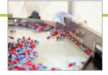
Proprietary Airguide System automatically sets pills onto a single layer and guides their flow into the center of the counting mechanism for proper presentation to the counting sensor.
