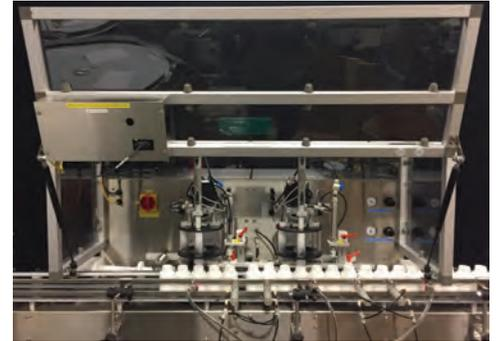
Comes with durable, clear, plastic safety shield. Opens for complete access to the interior, fast roll changeover.
