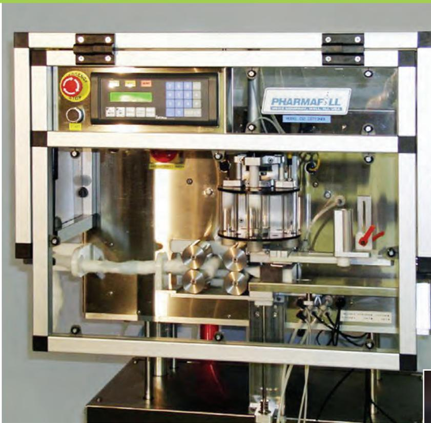
The Pharmafill CS2 Cotton Inserter automatically separates cotton, rayon and polyester from continuous rolls into individual pieces and inserts them into the center of bottles or other containers at speeds of up to 90 bottles per minute. It integrates many of the high-speed technology advances from the CS10 model with the economical advantages of the entry level CS1 model to offer speed, reliability and adjustable versatility all in one model.
