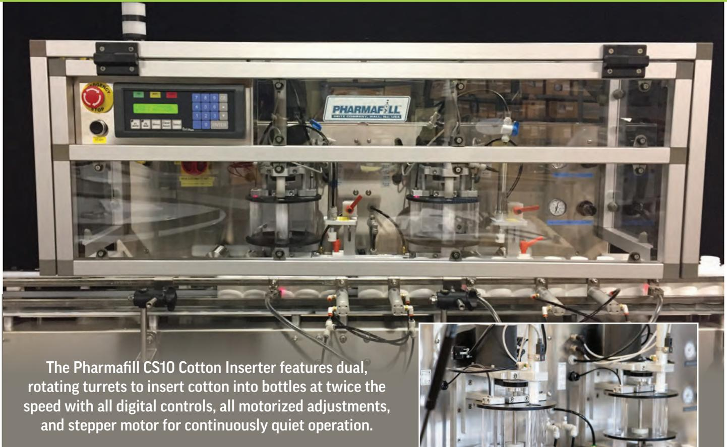
The Pharmafill CS10 Cotton Inserter features dual, rotating turrets to insert cotton into bottles at twice the speed with all digital controls, all motorized adjustments, and stepper motor for continuously quiet operation.
